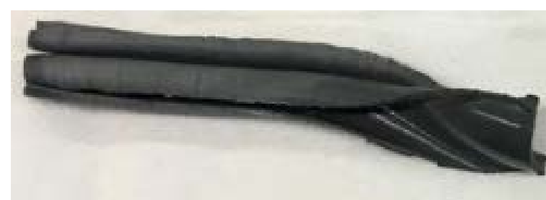
Figure 4: Warpage of PVC in acetone.
